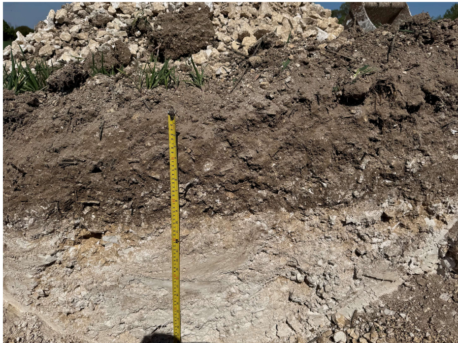
Image 3 – Pit 5, showing the grey silty clay loam topsoil over solid chalk layer at a shallow depth. By using the mini-digger, we were able to excavate pits deeper than would be possible by hand, to give a clear indication of this change in soil type and depth.
