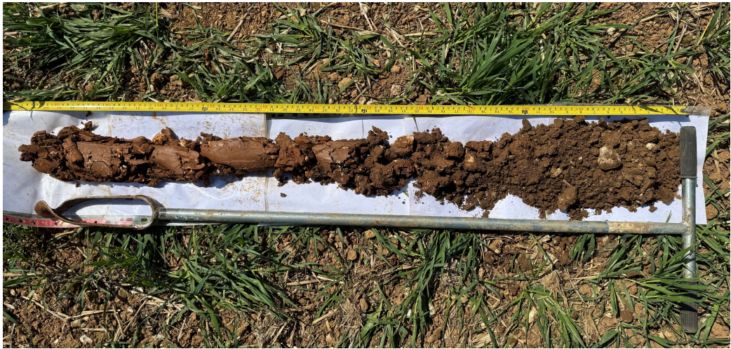
Image 2 – Boring 4, showing a brown, stony silty clay loam topsoil over a reddish brown stony silty clay subsoil – typical of Carstens. There was evidence of solid chalk beyond 120cm in places.
